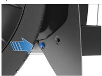
Install the opened (plastic rivet pulled out) new push clip into the outboard hole, and then push the plastic rivet in to close the push clip.
