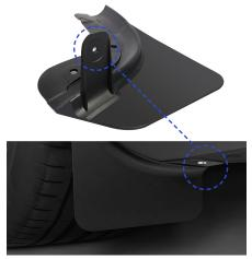
8. The installation of the rear mudflap is the same as that of the front mudflap, except that the bottom screw fixing hole is added. It is only necessary to remove the screws of the original car at the bottom before installing the mudflap, and then lock the screws of the original car after installing the mudflap.
