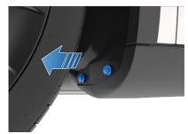
4. Maneuver the mud flap in place so that the tabs on the mud flap hook onto the backside of the front fender garnish. Make sure that the mud flap is aligned correctly with the holes in the front wheel arch liner and body of the vehicle.
