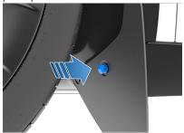
Perform this procedure again on the right side of the vehicle to install the right mud flap.
